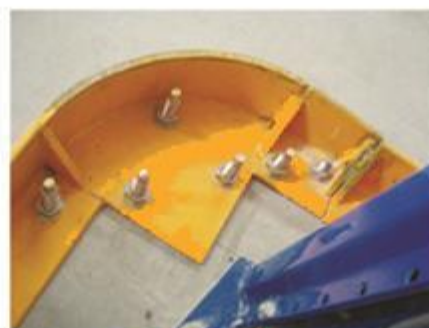
窄巷道护轨转角 VNA guide rail corner
